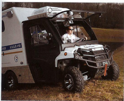
An Alternative Support Apparatus (ASAP) is an all-terrain vehicle that enables paramedics to reach patients in any terrain.
